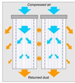
Left: Traditional cartridge filters suffer from reduced air flow towards the bottom as pressure is lost. There is also the serious issue of dust re-entrainment between neighbouring filters.
