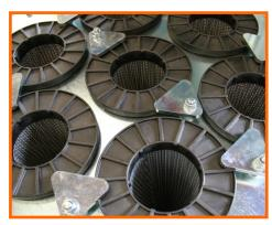
As shown in the illustrations below, this unique design means that 82% of the area at the inlet chamber of the filter unit is free, as opposed to a typical 59% when using cylindrical elements. This results in lower upward air velocities at this point, increasing dust separation. These features mean the filters have a longer functional life and offer a higher consistency of performance.
