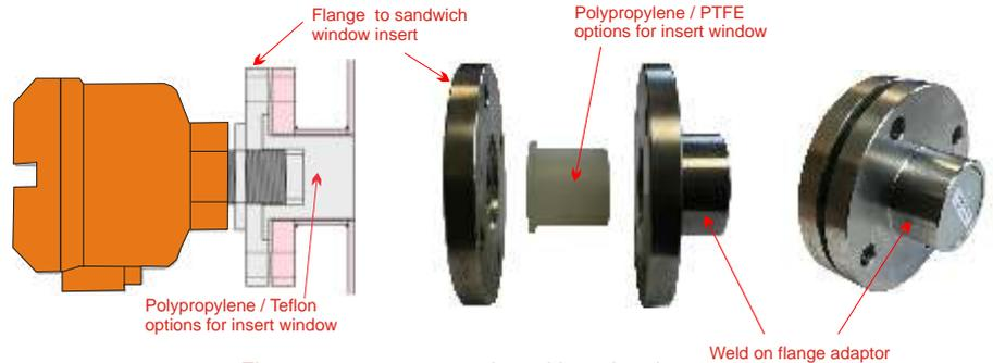
Flange process connection with optional polypropylene plug sandwiched between flanges but flush with pipe wall. This provides additional sensor protection.
