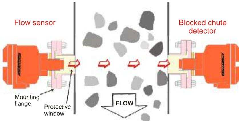
Combining the Microsense blocked chute detector with the Microsense flow switch provides a unique solution for two applications with one installation. For this application we utilise the flow switch on one side of the application and the receiver of the blocked chute switch on the other, as shown in the diagram opposite. This application would detect firstly if there is flow in the chute or pipe and secondly if the chute has blocked.
