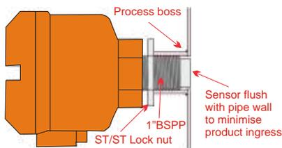
Standard G1 process connection connected directly into the pipe socket. Suitable for low abrasion applications.
